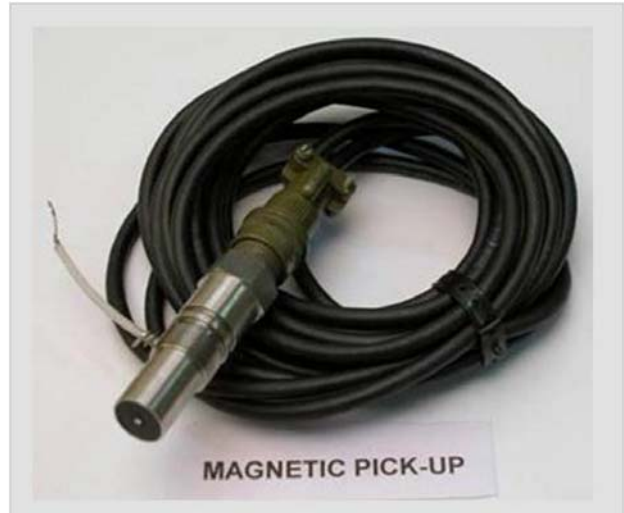
Fig. 8: Magnetic type speed pick-up
